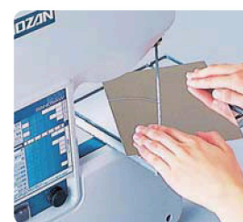
Cutting an aluminum sheet along a curved line
