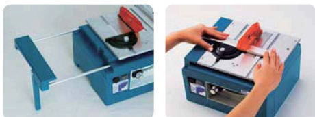
Max. table width of 500 mm when the table guide is extended
