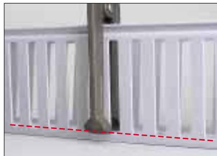
2. Cut the pillar with the outer side of the blade facing straight in front.
