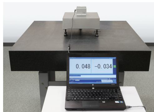
Output from sensors can also be displayed or recorded on PC with dedicated software.
