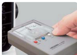
Ionizing air blower's ion balance adjustment
