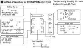
\* With Heater Breakage Alarm Function Type Only.
